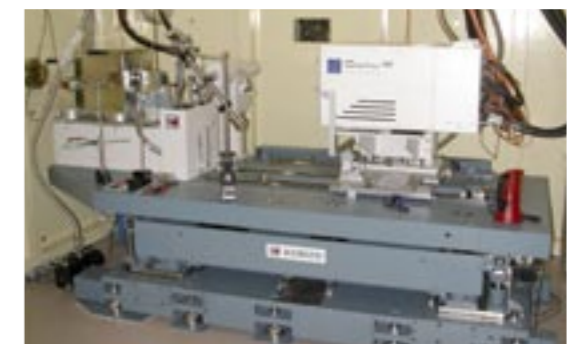
Large-area CCD detector and ultra-high precision diffractometer provided on BL-5
