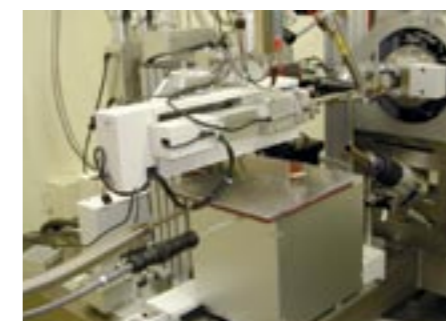
SPring-8 Precise Automatic Cryo-sample Exchanger (SPACE), a fully automated sample unit installed on the SPring-8 beamline BL26B2
