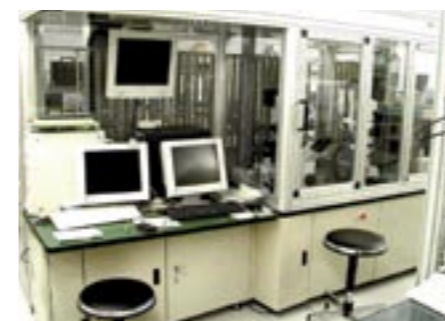
TERA, a fully automated robot that can search for crystallization conditions and observe crystal formation
